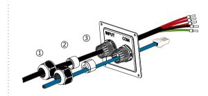
STEP 9: Insert the wires into the terminal blocks, then block the terminal with the straight screwdriver.
