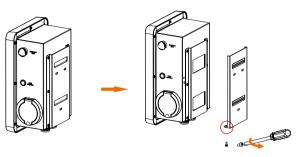
STEP 2: Fix the back bracket and the cable hook (only for type P) to the wall.
