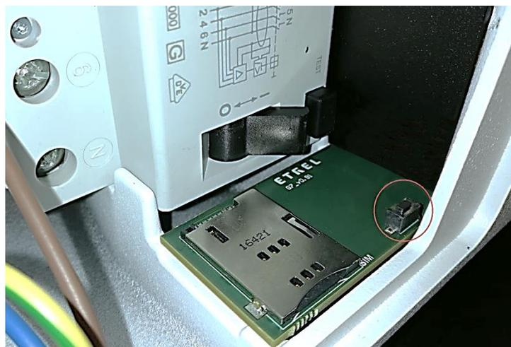
Figure 8: Reset button inside the maintenance opening
