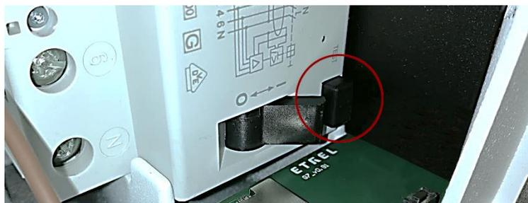
Figure 5: RCD test button
